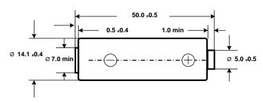
Dimensions are in millimeters and include label.
