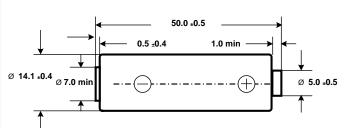
Dimensions are in millimeters and include label.
